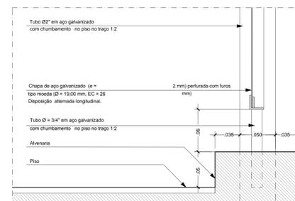
**13** DETALHE 10 - CORTE AA - DETALHE BASE GUARDA-CORPO
