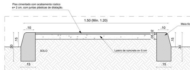
**08** DETALHE 05 - CORTE TÍPICO TRANSVERSAL DA CALÇADA - MEIO FIO
