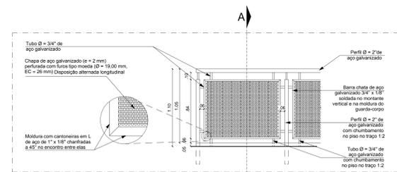
**09** DETALHE 06 - VISTA INTERNA - DETALHE DO GUARDA-CORPO
